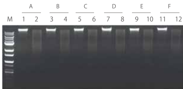
Lane M : 1 kb Labo DNA ladder Lane 1, 3, 5, 7, 9, 11 : Purified genomic DNA from human whole blood Lane 2, 4, 6, 8, 10, 12 : Restriction enzyme digestion (HindIII) of purified genomic DNA from human whole blood
